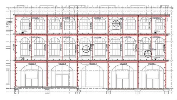
The new steel frame was attached to the façade with anchors being spaced at approximately 1 metre centres either horizontally or vertically.
