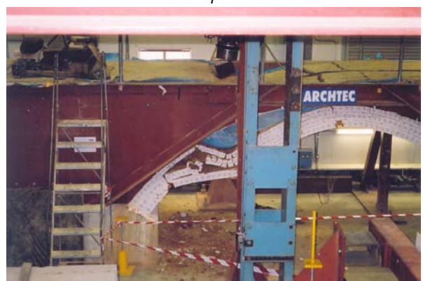
Figure 9.1 Failure of strengthened arch observed in the second Archtec test at TRL (Note that between each stage the arch remains stable under a minimum of its own self weight and further load/displacement had to be applied via the jack to progress the failure)
