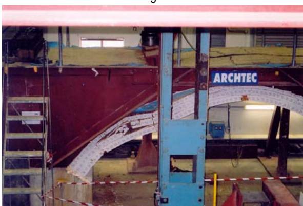
Figure 9.1 Failure of strengthened arch observed in the second Archtec test at TRL (Note that between each stage the arch remains stable under a minimum of its own self weight and further load/displacement had to be applied via the jack to progress the failure)
