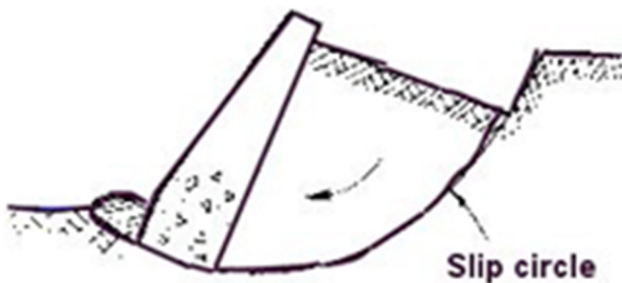
Deep seated failure
