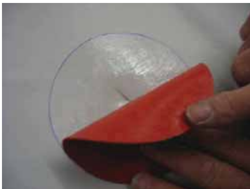
Once the second coat has become touch dry (about 2 mins.) place over the tear.
