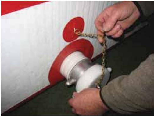
Unscrew protective caps from external male 4" fittings
