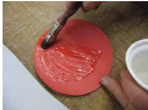
Apply glue to the patch. Wait 20 minutes and apply second coat
