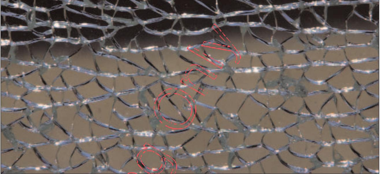
*There are several means of treating windows for blast-resistance. While window film is the most cost-effective option, it cannot withstand high blast-loads. Although ballistic glass can be a tougher choice, its thickness and rigidity need strongly built anchors. It could also possibly require wall reinforcement.*
