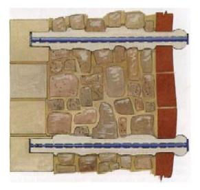
anchors were installed from the inside of the building. They were allowed to project into the building to permit the standard circular crimped anchor body. The anchor projection was cut off flush internally and plastered over.
