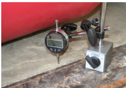
Deflection being measured against load applied.
