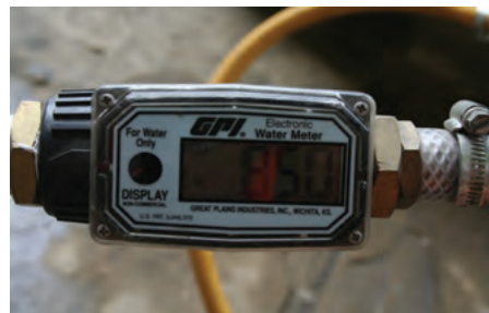
Flow meter measuring water in bag.
