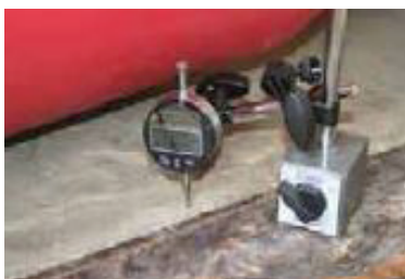
Deflection being measured against load applied.
