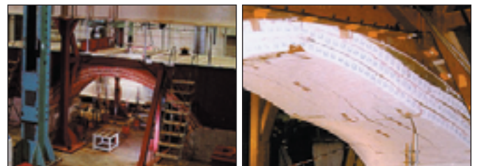
Figure 4. Full-scale masonry arch tests at the TRL
