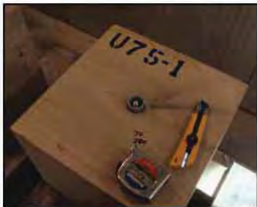
(e) External PVC Confinement within Hole
