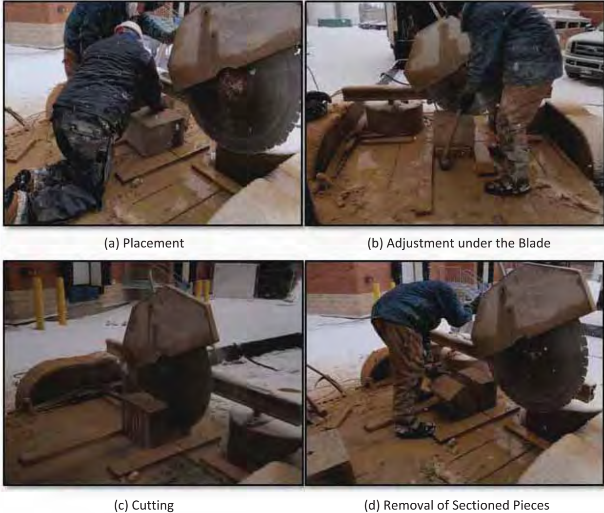
Figure 16 – Sectioning Procedure (DiTECH International Inc.)
