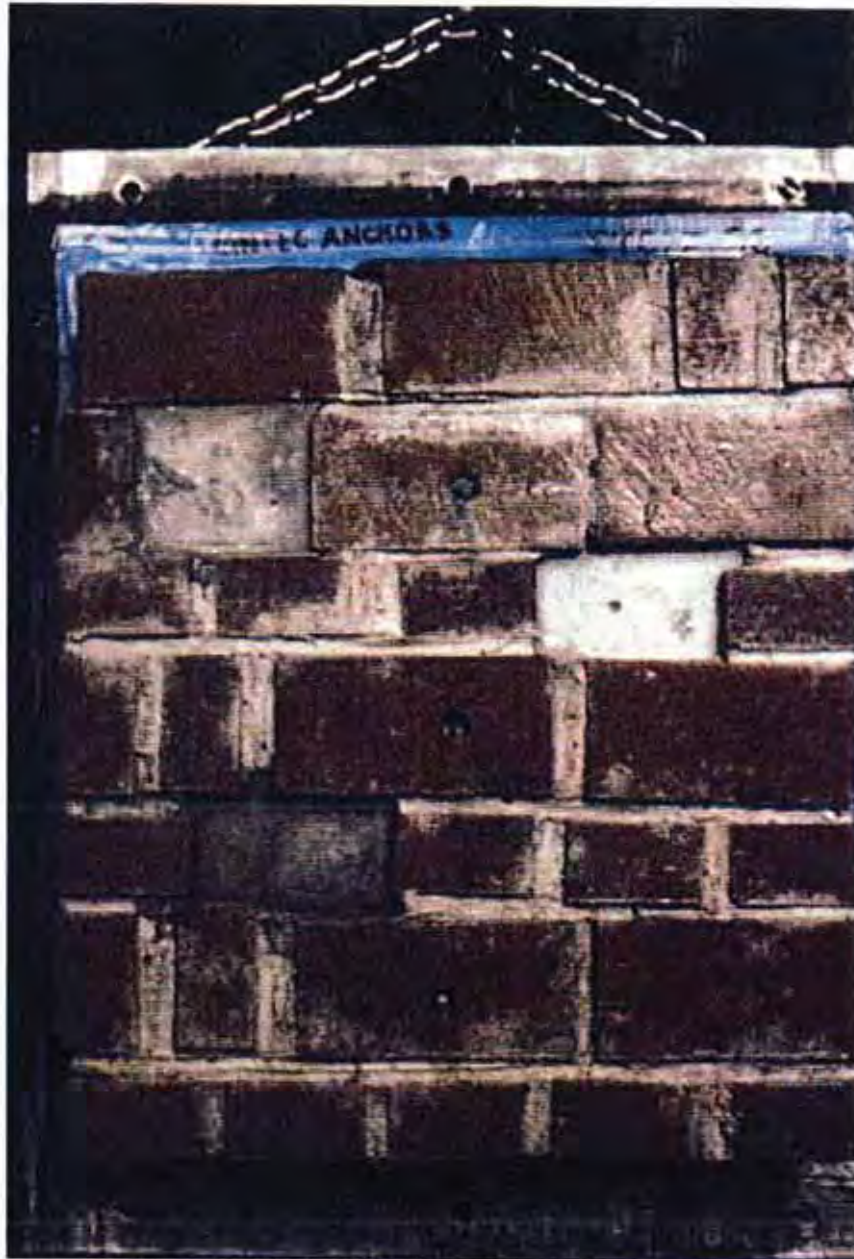
Figure 4 Wallette A after 100 freeze-thaw cycles
