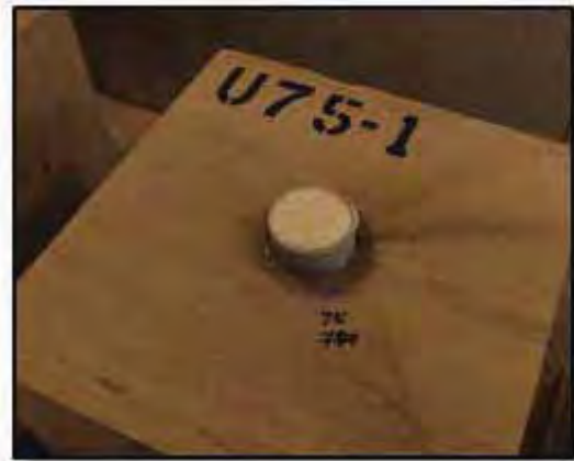
(h) Insulating Foam against Moisture Ingress (Expansive Insulating Foam Used)
