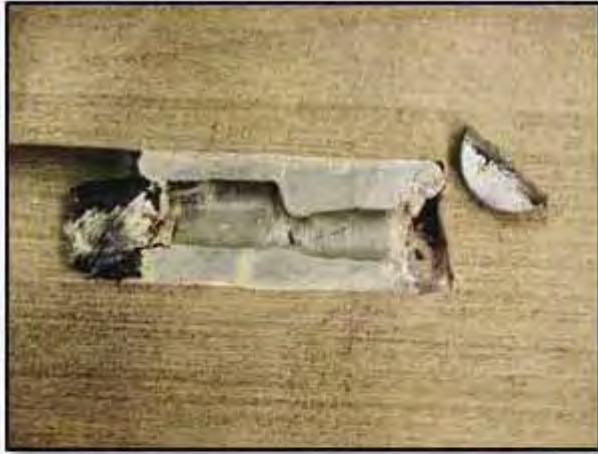
Figure B.5 – Wet Freeze-Thaw Samples (75mm Sock Length)
