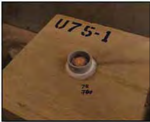
(g) External PVC Confinement on the Stone Surface (Silicon added to Seal the Hole)
