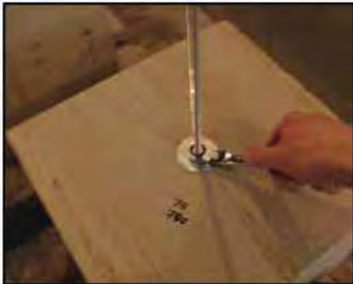
(c) Rod Stabilization (2"OD -3/8"ID Washer & Nut)
