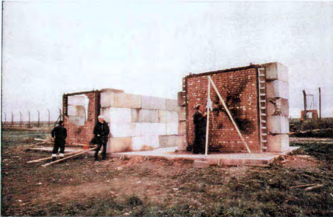
Fig. 1 – Post test results of the first Blastec Wall Trial – 8 Nov 99. Two identical 225mm (9”) thick masonry walls each subjected to a blast load of 7.8kg (18.1lbs) TNT NEQ at 1m (3.25’). The wall on the left was unreinforced; the other reinforced by Cintec “Multibar Anchors” at 225mm (9”) vertical centres.
