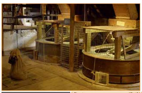
Nether Alderley Mill The machinery at the mill is over 100 years old, with some parts dated to 1871. The millstones weigh over a ton and our technicians secured the old mill stone to the floor using 4 x 1m anchors to ensure it was safe when the public visited.
