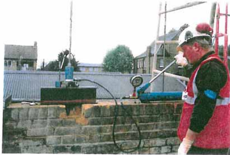
Figure 4 Post-tensioning Anchor in Test Panel
