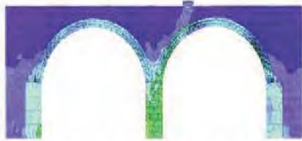
Typical test simulation illustrating principal compressive stresses; blue, green and yellow reveal increasing levels of compression
