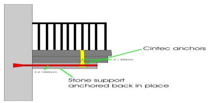
The diagram above shows a 1300mm Cintec anchor installed in a 50 mm hole profiled out to 65 mm over the bottom 250 mm, together with a 350 mm Cintec anchor installed in a 50 mm hole profiled to 65 mm over the last 200 mm.
