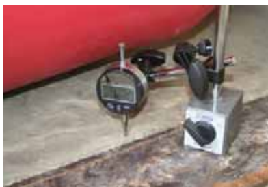
Deflection being measured against load applied
