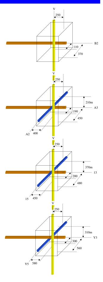
Anchor positions were carefully marked out and drilled with extreme precision to avoid intersecting anchors.
