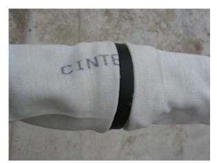
Cintec Multibar anchors Comprising two 25mm ribbed stainless steel bars were assembled in sections to achieve anchor lengths up to 29 metres. Each anchor had integral plastic spacers, to ensure centralisation of the anchor along its length, within the drilled hole.
