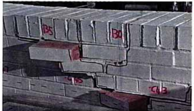
Although the bridge was shunted by the force of the impact, it remained intact with no significant spalling. The picture above shows the wall face opposite to the point of impact after two consecutive tests.
