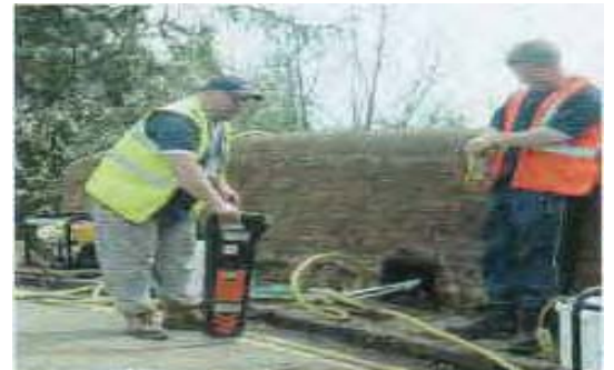
Checking for sub-surface services during bridge survey
